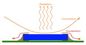
**The Rated Power** of a resistor depends on the maximum available heat transport capability, which mainly relies on heat conduction through the solder joint to the PCB. The temperature dissipation through air convection and radiation can be neglected. The WU73 flat chip resistor use the long sides of the resistor to give better heat dissipation through the solder junctions.
